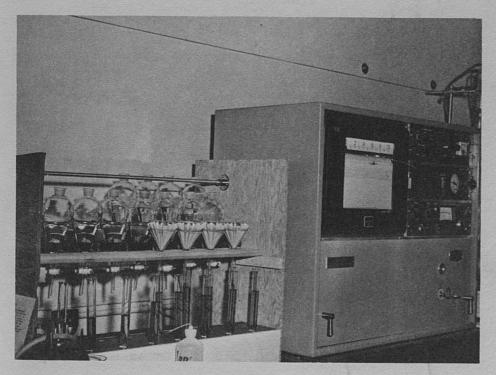
Residues of insecticides are analyzed by gas chromatography, using the equipment shown here.
