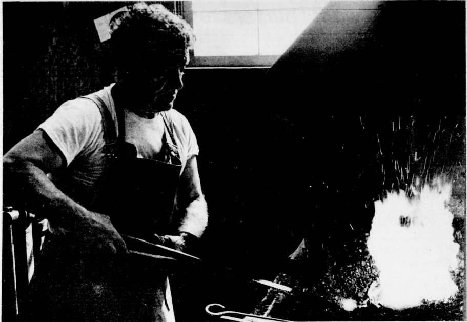
The farrier at his forge is a familiar sight at the Horse Park. Above, Roberts fires up his forge and places an unformed shoe in the hot coals. After removing it from the fire, it will be formed for a particular horse.
