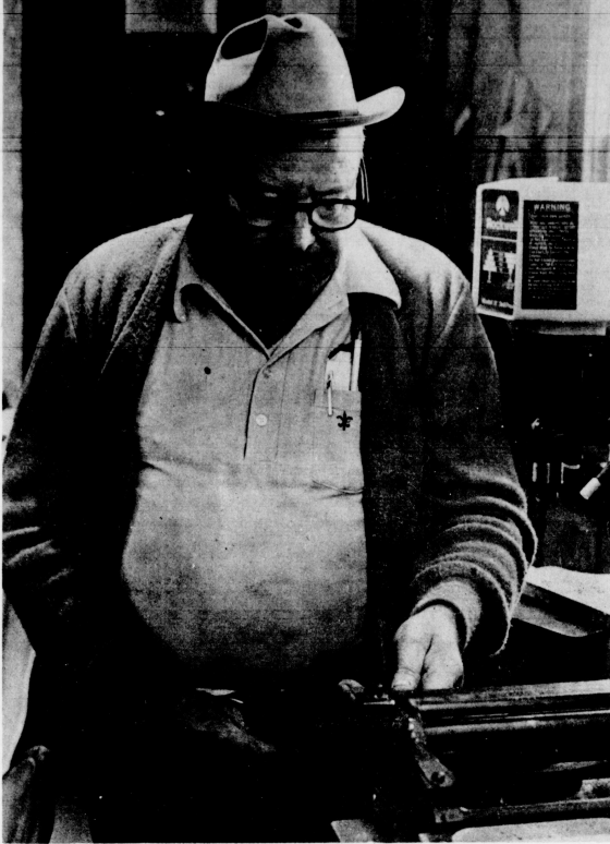
Before leather can be cut and patterned it sometimes has to be thinned down. Roush prepares to pull a piece of leather through a special lathe to give him the correct width.
