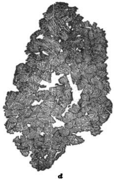
MICROSCOPIC STRUCTURE OF THE TRENTON LIMESTONE.
