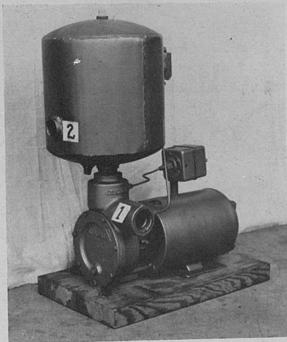
FIGURE 8. A centrifugal pump for shallow-well operation. 1. Suction pipe connection. 2. Discharge pipe connection.
