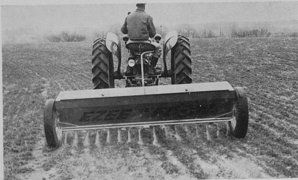
Fig. 9.— Use of a hopper spreader drawn by a tractor is a good way to spread limestone evenly.
