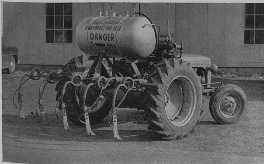
Fig. 1.—A tractor-mounted anhydrous ammonia applicator equipped with a pump-type metering device and five spring-tine mounted applicators.
