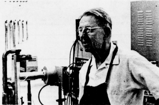
Karl Schneider, an instrument maker at UK for 45 years, is shown with the scattering chamber he built. This chamber is for the Van de Graff accelerator located in the silo of the Chemistry-Physics Building.
