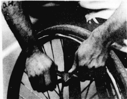
Stresses in cornering and opponents footsteps can snap the spokes.
